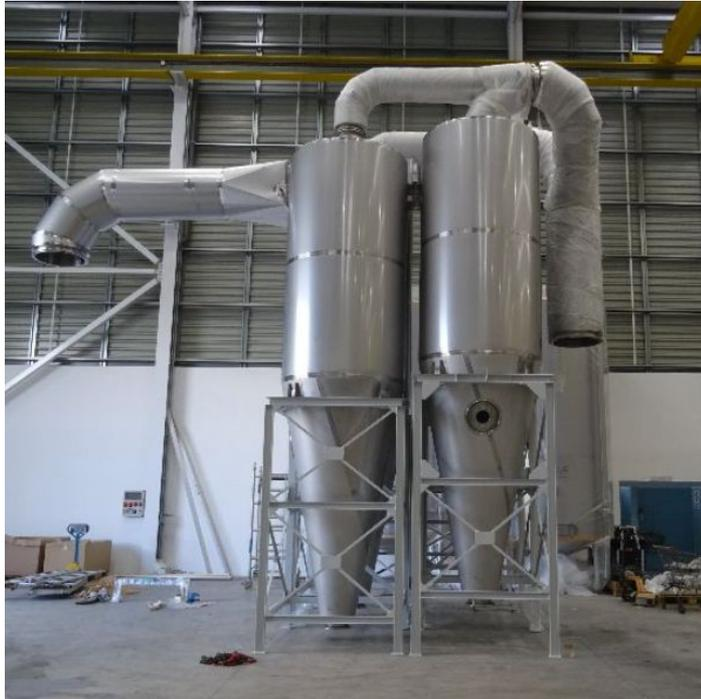
The 4 Hurricane RE cyclone system is ready to ship and install at the client's plant. This is planned for next month. The cyclone set will control emissions and recover product in a Norwegian plant that manufactures fish and seafood flavors.
