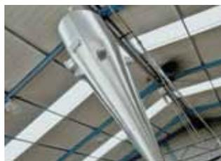
**Hurricane HR** optimized cyclone for API recovery after a mixer with 3,400 Am<sup>3</sup>/h flow rate @ 75 °C. The cyclone is ø 800 mm, manufactured in AISI 316L under the most strict pharmaceutical quality standards.
