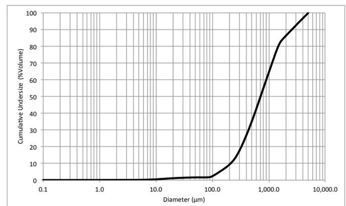
Fig. 2 – Particle Size Distribution used in simulations
