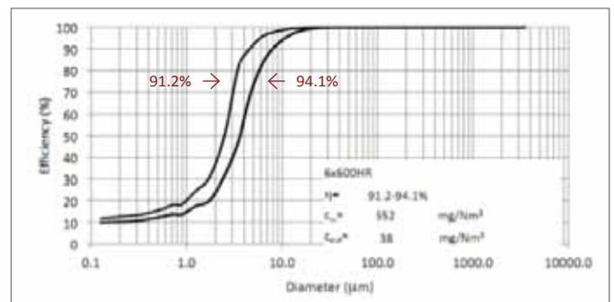
Fig. 4 – Predicted grade and global efficiency for hurricane system (KT).
