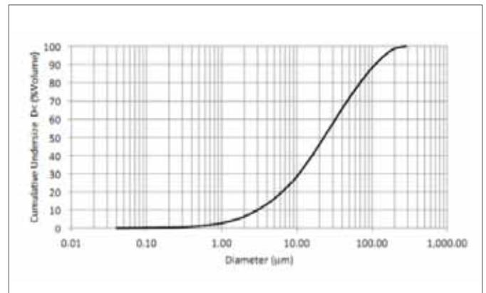
Fig. 3 – Particle size distribution used in simulations for JT (Coulter laser analyser).
