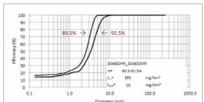
Fig. 5 – Predicted grade and global efficiency for ReCyclone MH system (JT boiler).
