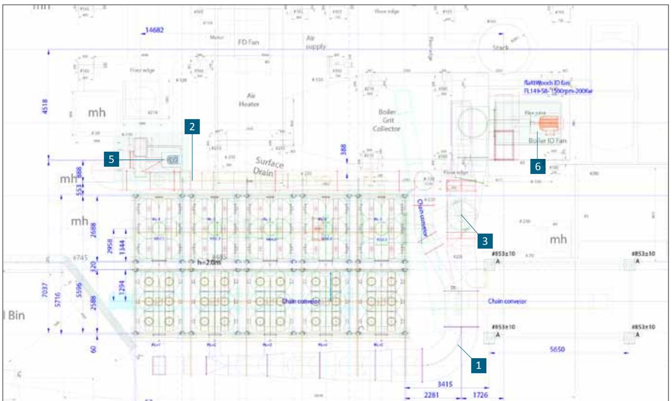
Fig.7 - Drawing of ReCyclone MH System: 1. Inlet Ductwork | 2. Recirculation Ductwork | 3. Outlet Ductwork | 4. Rotary Valves (not visible) | 5. Recirculation Fan | 6. Exhaust Fan
