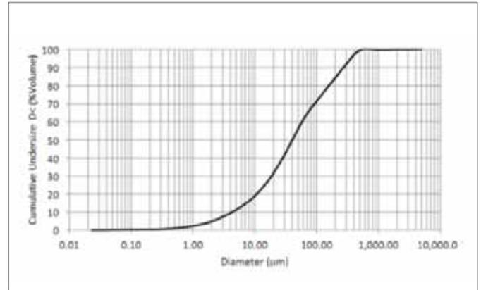
Fig. 2 –Particle size distribution used in simulations for KT (Coulter laser analyser).
