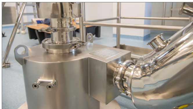
Fig 4 & 5 - Gas inlet (from Spray Dryer) and Gas outlet (to bag filter)
