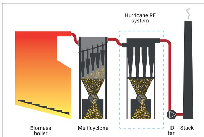
Fig. 1 – Process flow diagram from existing installation
