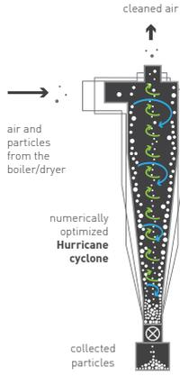
**Hurricane** cyclones are patented numerically optimized cyclones. **Hurricane** geometries maximize powder collection for each different application, while minimizing reentrainment and keeping pressure drop at reasonable levels. Hurricane cyclones demonstrate impressive efficiencies in capturing very fine powders with a Volume Median Diameter (VMD) of less than 5µm.
