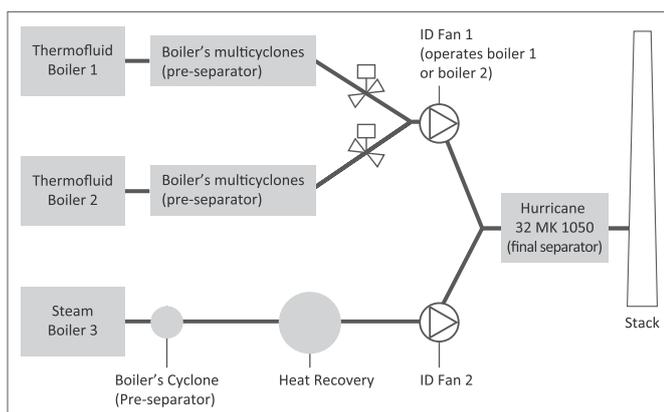
Fig. 1 – Process Diagram
