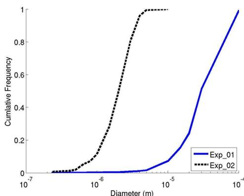
Fig. 11 – Cumulative Particle Size Distributions
