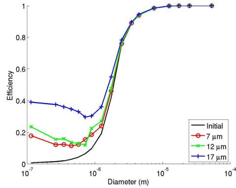
Fig. 9. Cutoff-diameter influence: 10 ms, 1500  $\text{kg}/\text{m}^3$ , 700 $\text{mg}/\text{m}^3$ , 5 slices
