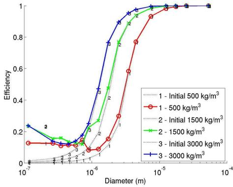
Fig. 7. Specific gravity influence: 10 ms, 6  $\mu\text{m}$ , 700  $\text{mg}/\text{m}^3$ , 5 slices
